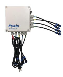
A typical setup procedure involves the user connecting one ST-500 sensor, one ST-720 sensor and one ST-712 sensor to the sensor input glands 1, 2 and 3 (bottom) and then connects the output cable from 4-20mA signal glands 1,2 and 3 (right) to controller 4-20mA input channels. The last step is to connect the power plug to the power outlet. PowerPack comes with standard 110V USA plug adapter, however, unit is fully functional with 240VAC operation using a standard outlet conversion adapter.
